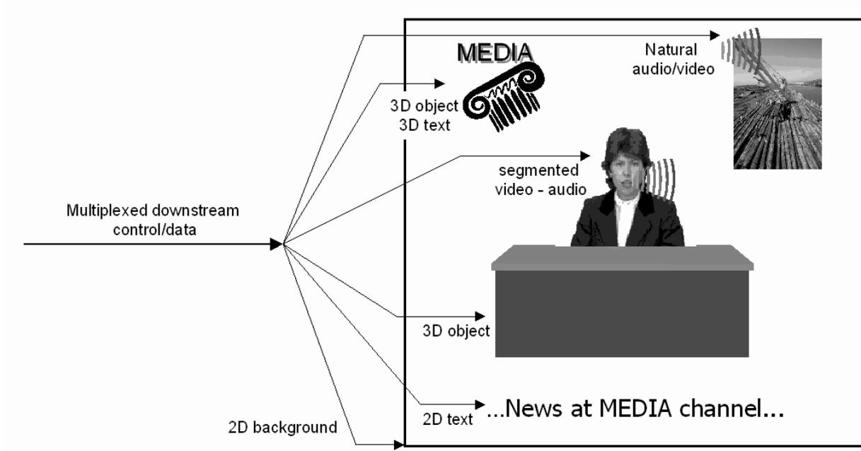
Fig. 4. Example of an MPEG-4 scene.
