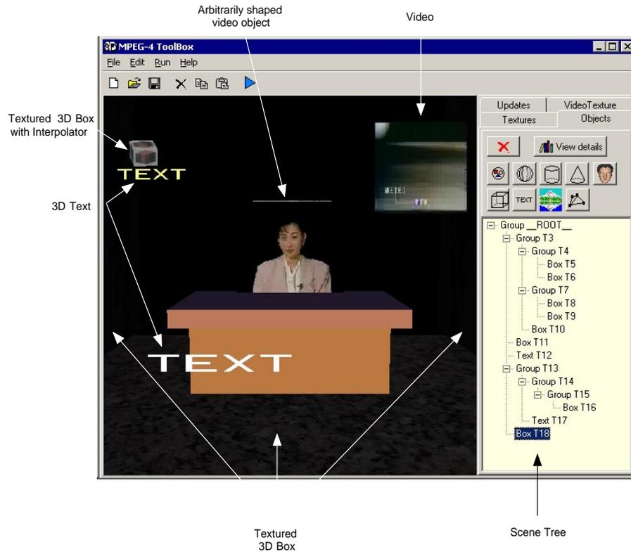
Fig. 20. The virtual studio scene using arbitrarily shaped video objects in the authoring tool.
