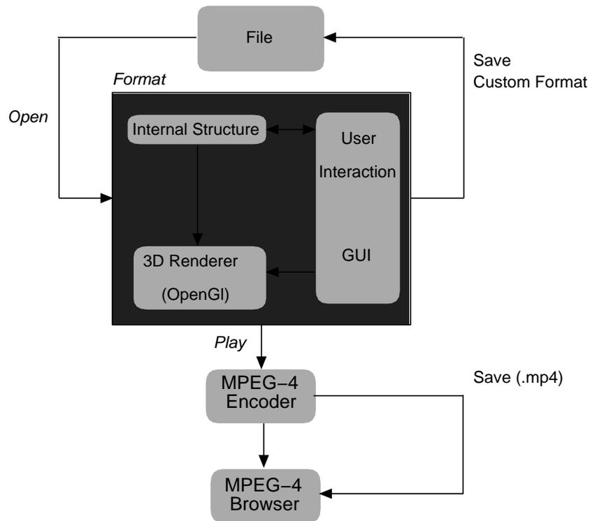
Fig. 7. System Architecture.
