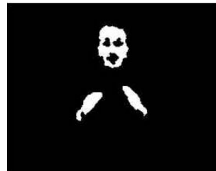
Figure 15. Closing of Figure 14, final color mask
