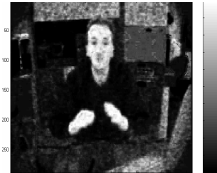
Figure 19. Moving hand segments after morphological reconstruction
