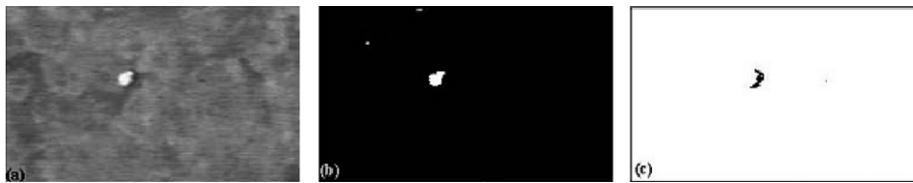
Fig. 5. (a) Sub-region of an image illustrating a sheltered fluting cleaned by the Biological Paste method (BP), (b) white and (c) black particles detected by the MFD algorithm.
