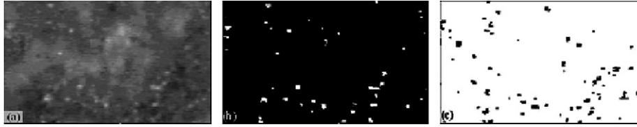
Fig. 4. (a) Sub-area of an untreated black crust located on fluting at sheltered areas, (b) white and (c) black particles detected by the MFD Algorithm.
