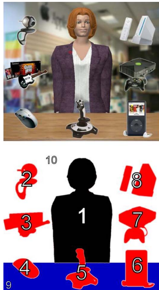
Fig. 3 Depiction of ( top ) the scenario, containing the Greta agent [16], acting in the role of a salesperson, and a number of objects and ( below ) the contents of the scene depicted in terms of virtual attention objects (VAO's). Each VAO records when and to what degree the user has been looking at it
