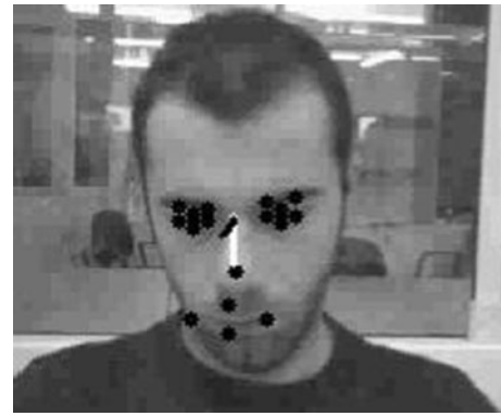
Fig. 1 Gaze direction detection is based on a number of tracked features (shown here as black dots ) in order to calculate a final head pose ( white line ) and eye gaze ( black line ) vector
