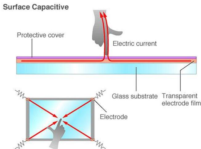
Figure 4.14 Surface capacitive touch screen
