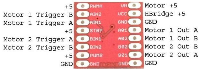
**Figure 4.9** Pin layout of the motor controller TB6612FNG
