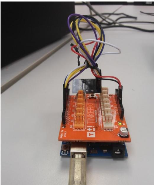
**Figure 4.15** The (server) Arduino Uno, connected with the RF antenna
