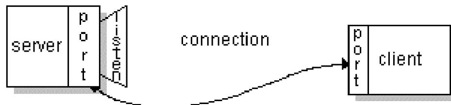
exception is thrown. **Figure 4.19** Server accepting the client's request and establishing a connection
