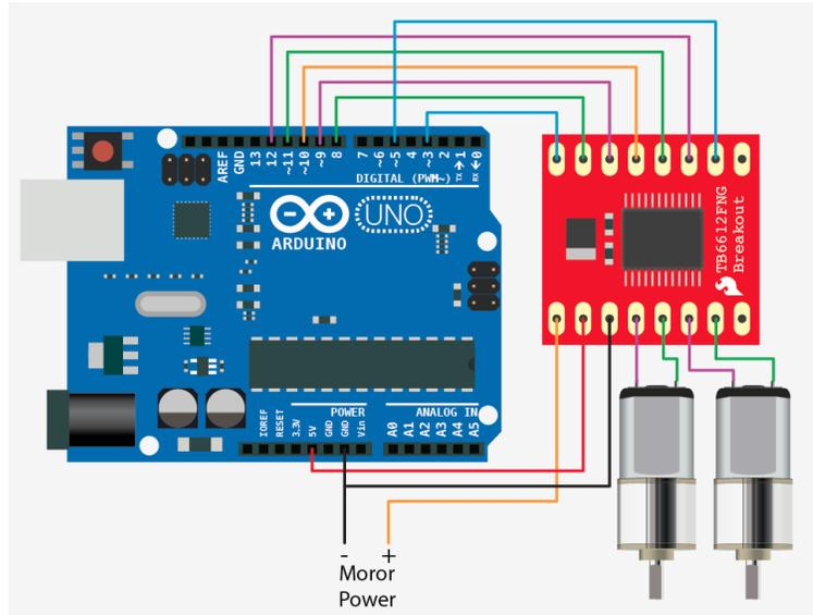
**Figure 4.11** Indicated connections between Arduino and motor controller
