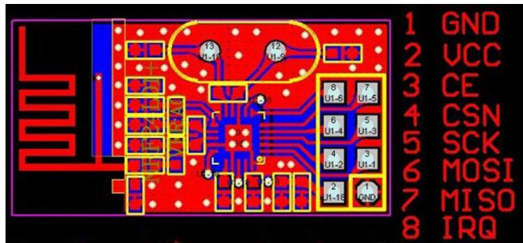
**Figure 4.12** Pin allocation of the RF antenna
