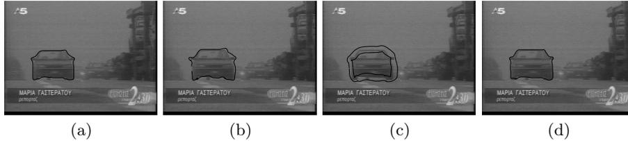
**Fig. 2.** Tracking method in steps: (a) object contour in the previous frame, (b) snake initialization in the current frame, (c) uncertainty region, (d) object contour in the current frame.
