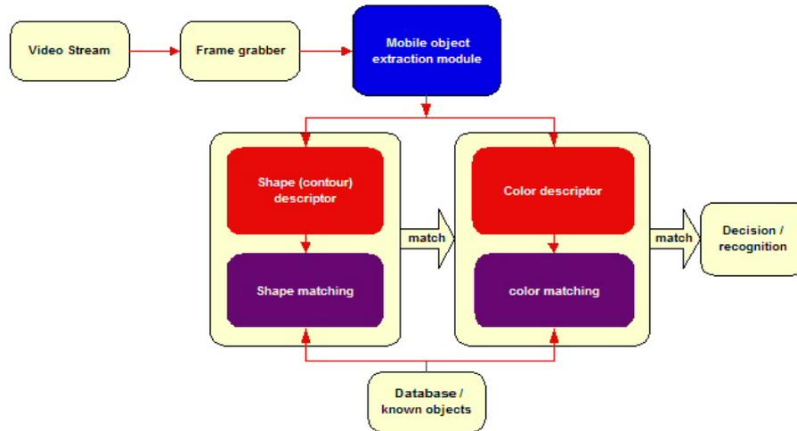
**Fig. 1.** The proposed integrated scheme for object recognition, using the shape and color descriptors.
