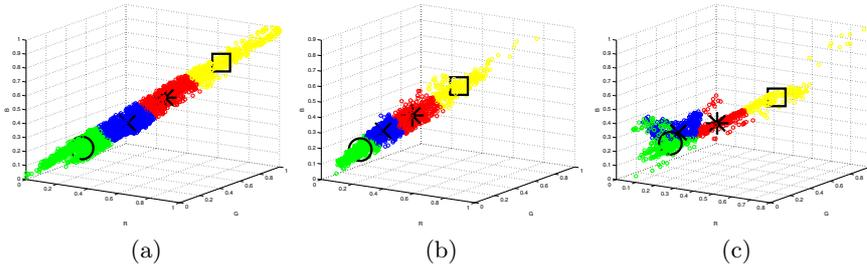
**Fig. 9.** Color distributions for the three objects, in the  $RGB$  space, after clustering: four color clusters for each object have been estimated, whereas the center of each cluster is also illustrated.
