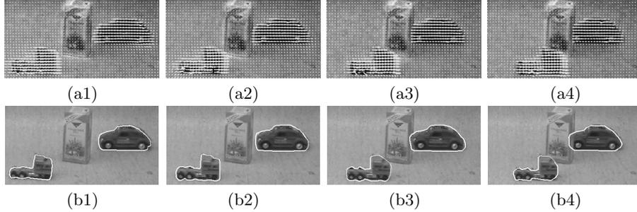
**Fig. 3.** (a1)-(a4) Motion estimation results and (b1)-(b4) the respective tracking results for a case of two moving objects.
