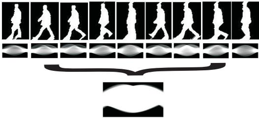
**Fig. 2.** Extracted silhouettes and Radon transforms for one walking period. History Trace template is shown on the bottom.
