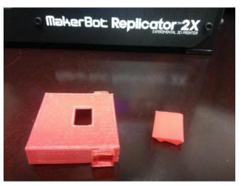
Figure 4.4 Our car parts (platform and bumper) after printing
