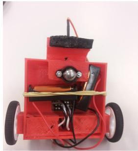
Figure 5.1 View of our car from below. We can observe the presence of the two batteries and the 'free wheel' that replaces two conventional front ones.
