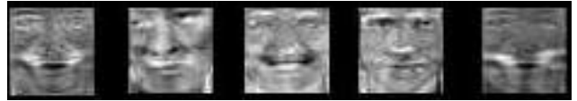
Fig. 4 Weights of five hidden layer neurons of a MLP-network of size (1295x5x4) for recognizing the facial expressions neutral, angry, happy, and sad.
